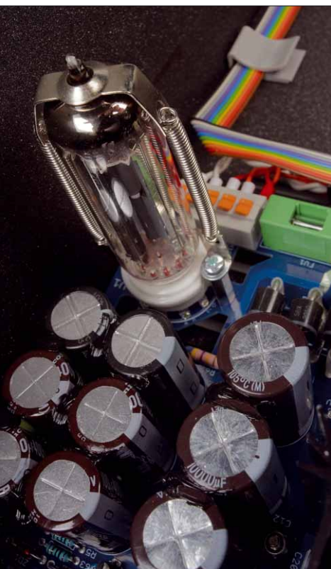
An EZ81 is used as the rectifier tube
