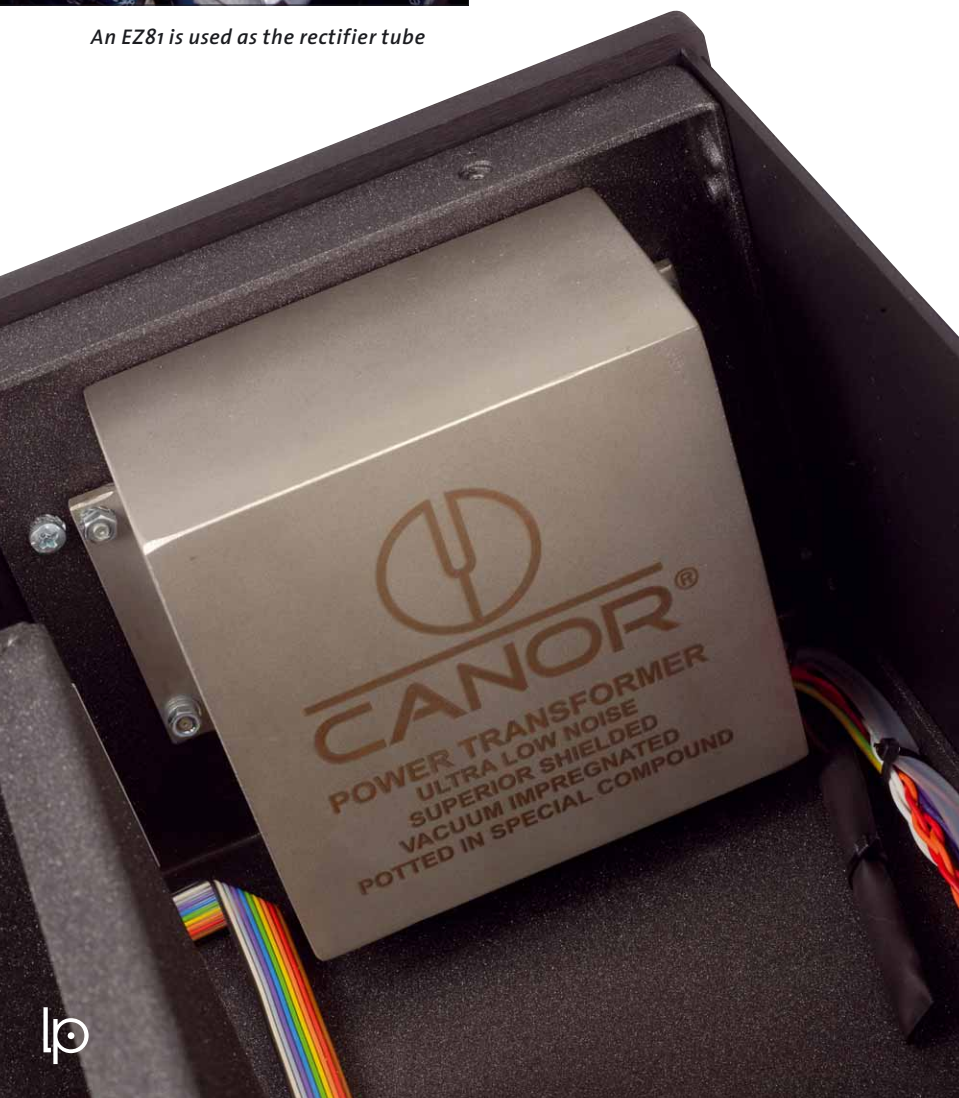
The thoroughly encapsulated toroidal transformer is located behind the front panel
